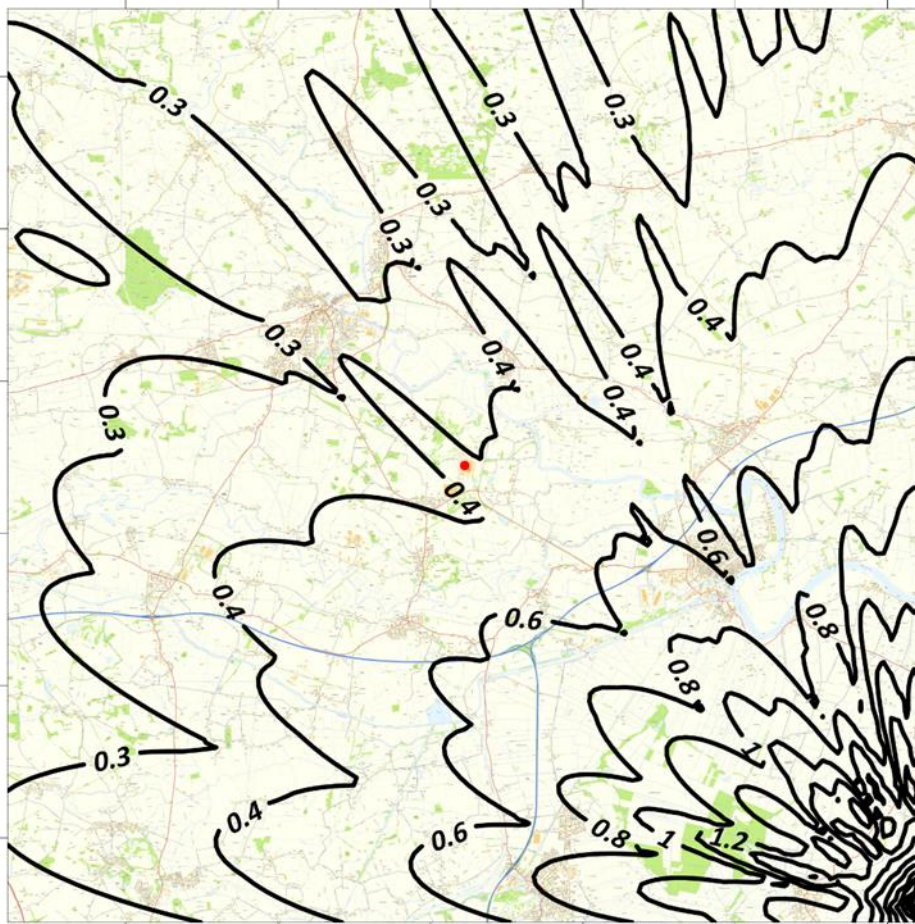
Plate 3-4 - Maximum hourly mean cumulative amine impacts (Proposed Scheme plus Keadby) for 2016. Drax Power Station is shown by the red circle. Concentrations shown in \mu\text{g}/\text{m}^3 . The degradation of amines is neglected in the modelling.
